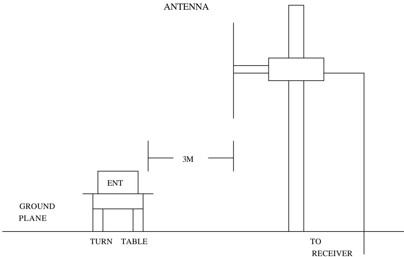
**4 . 3 RADIATED TEST SET-UP**
