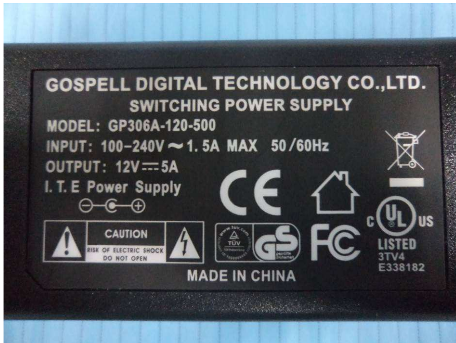
EUT – Adapter Label View
