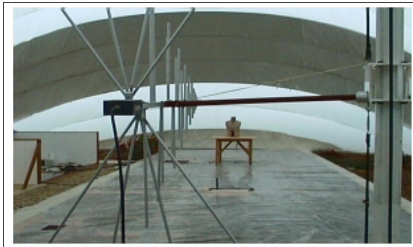
Fig.2 EUT on 10-m OATS for radiated RF emission testing.
