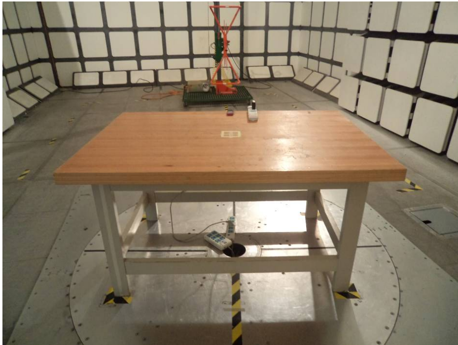
Radiated Emissions – Rear View (Charging & Playing mode)
