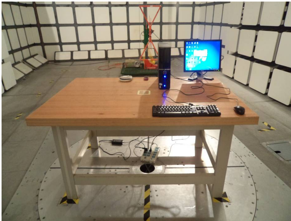
Radiated Emissions – Rear View (Downloading mode)
