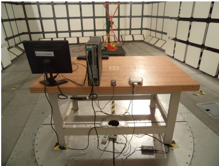
Radiated Emissions – Rear View (Downloading mode)
