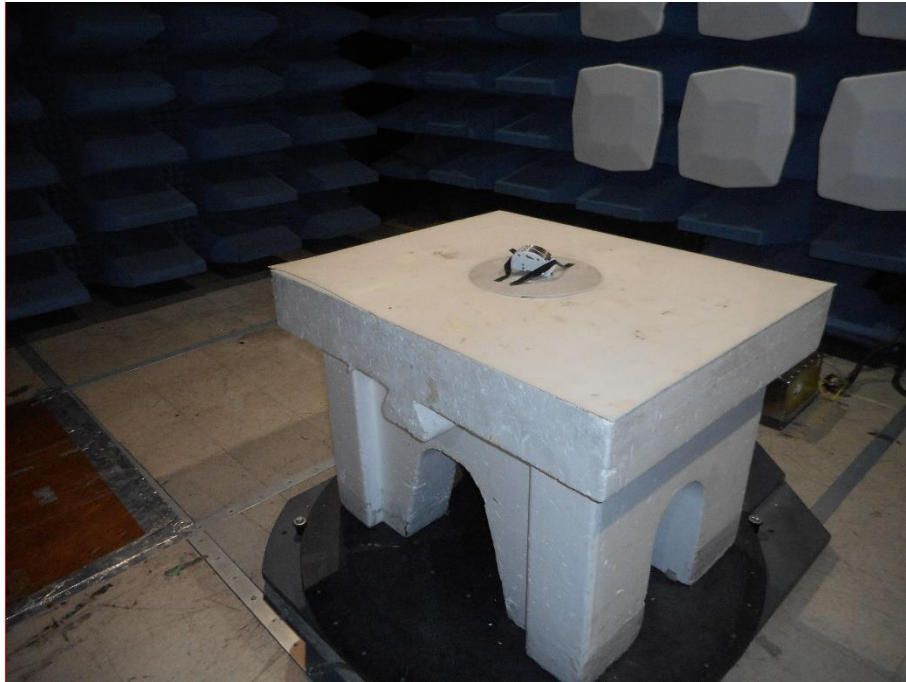
Figure3: Intentional Radiated Emissions performed at the 3m SAC, 30MHz – 1GHz, the EUT setup
