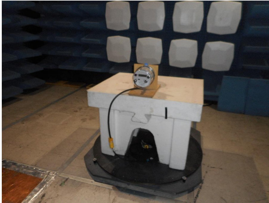
Figure 7: Unintentional Radiated Emissions performed at the SAC (close-up view) Test Setup: 4 models
