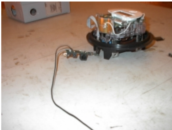
Emissions Test Setup Side View Showing Antennas O on Bottom
