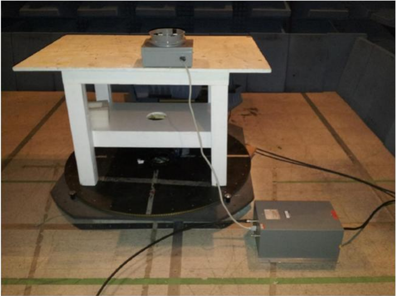
Figure 35: AC Conducted Test Setup
