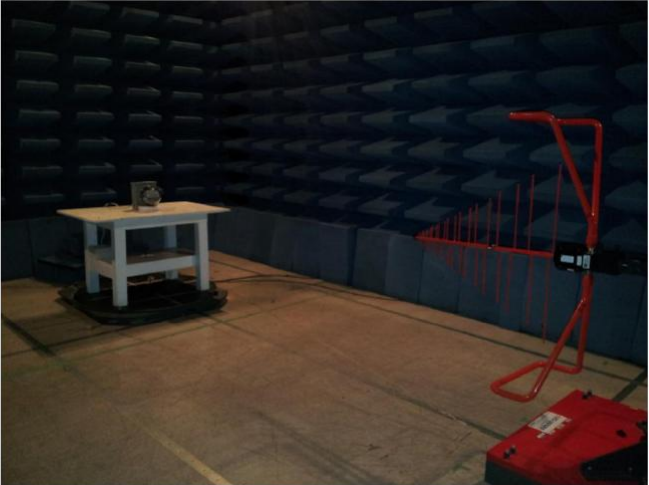
Figure 36: Emissions Test Setup – Intentional / Unintentional Radiated Emissions
