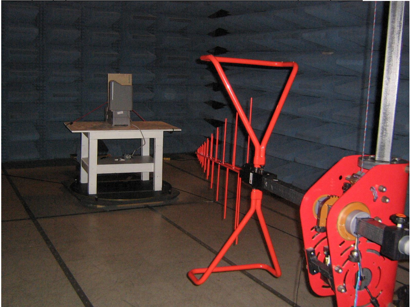
Intentional / Unintentional Radiated Emission 30 – 1000 MHz setup
