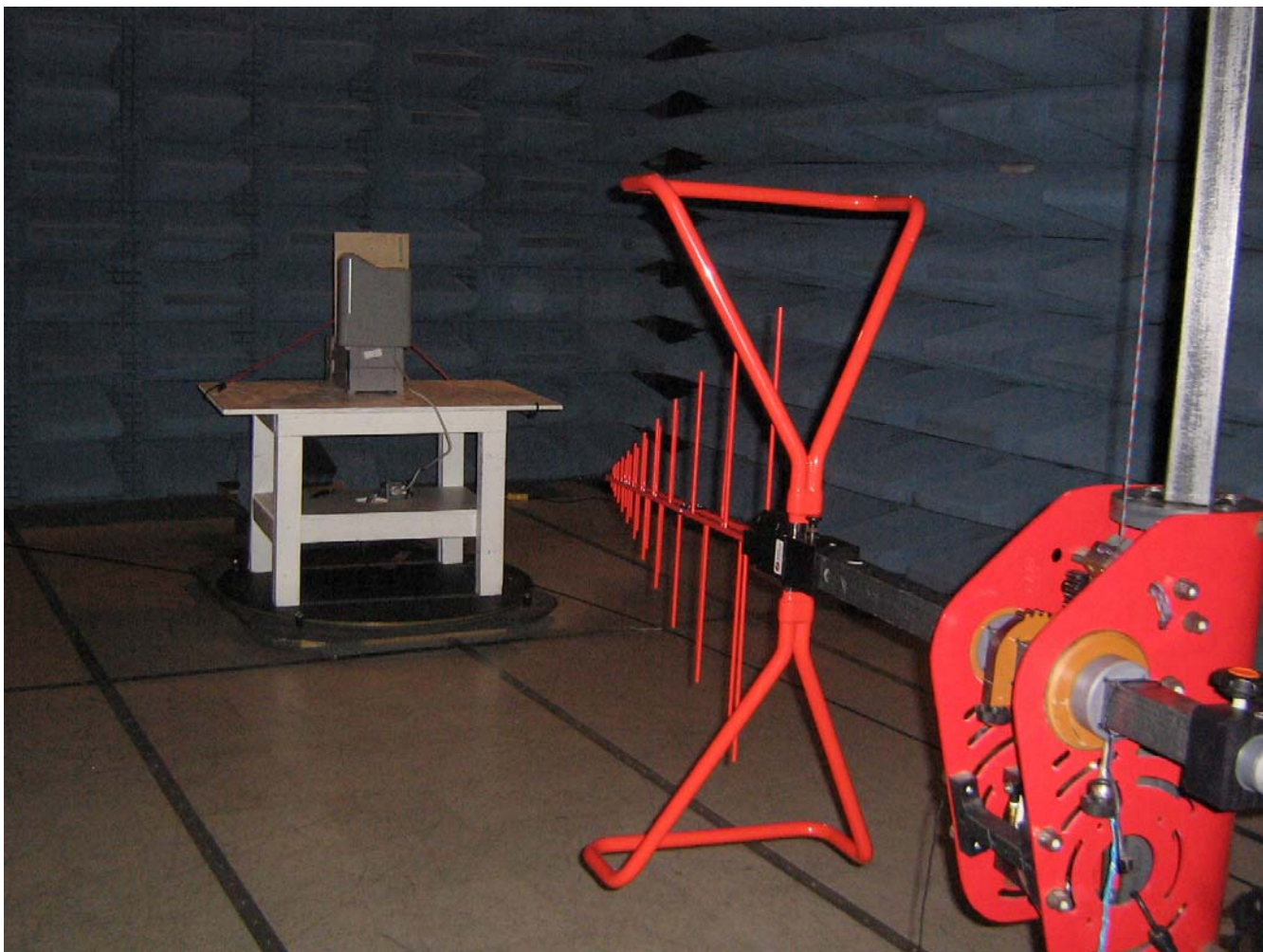
Emissions Test Setup – Intentional / Unintentional Radiated Emissions 30 – 1000 MHz
