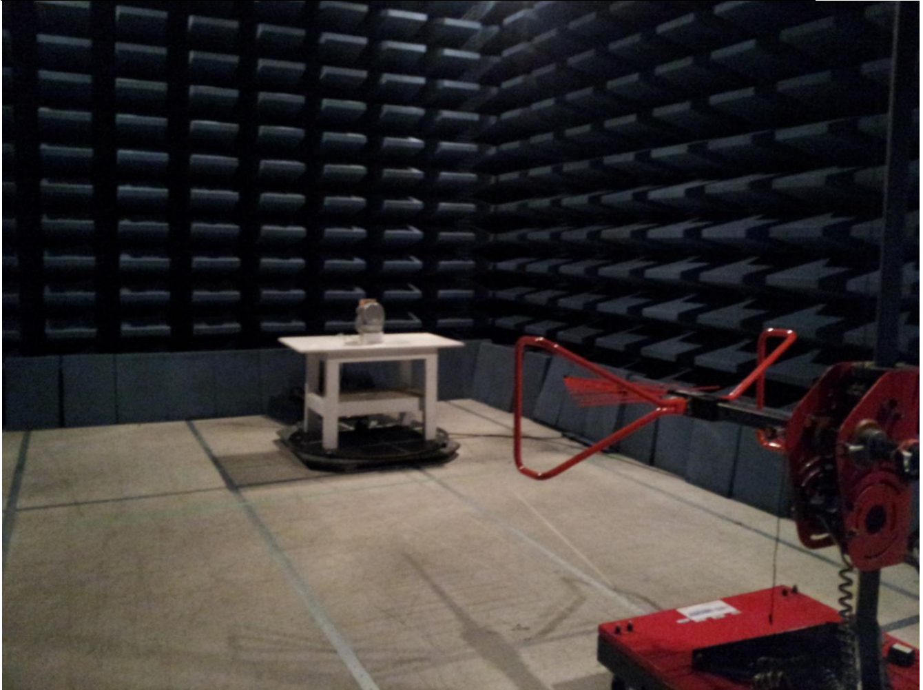
Figure 19: Emissions Test Setup – Intentional / Unintentional Radiated Emissions
