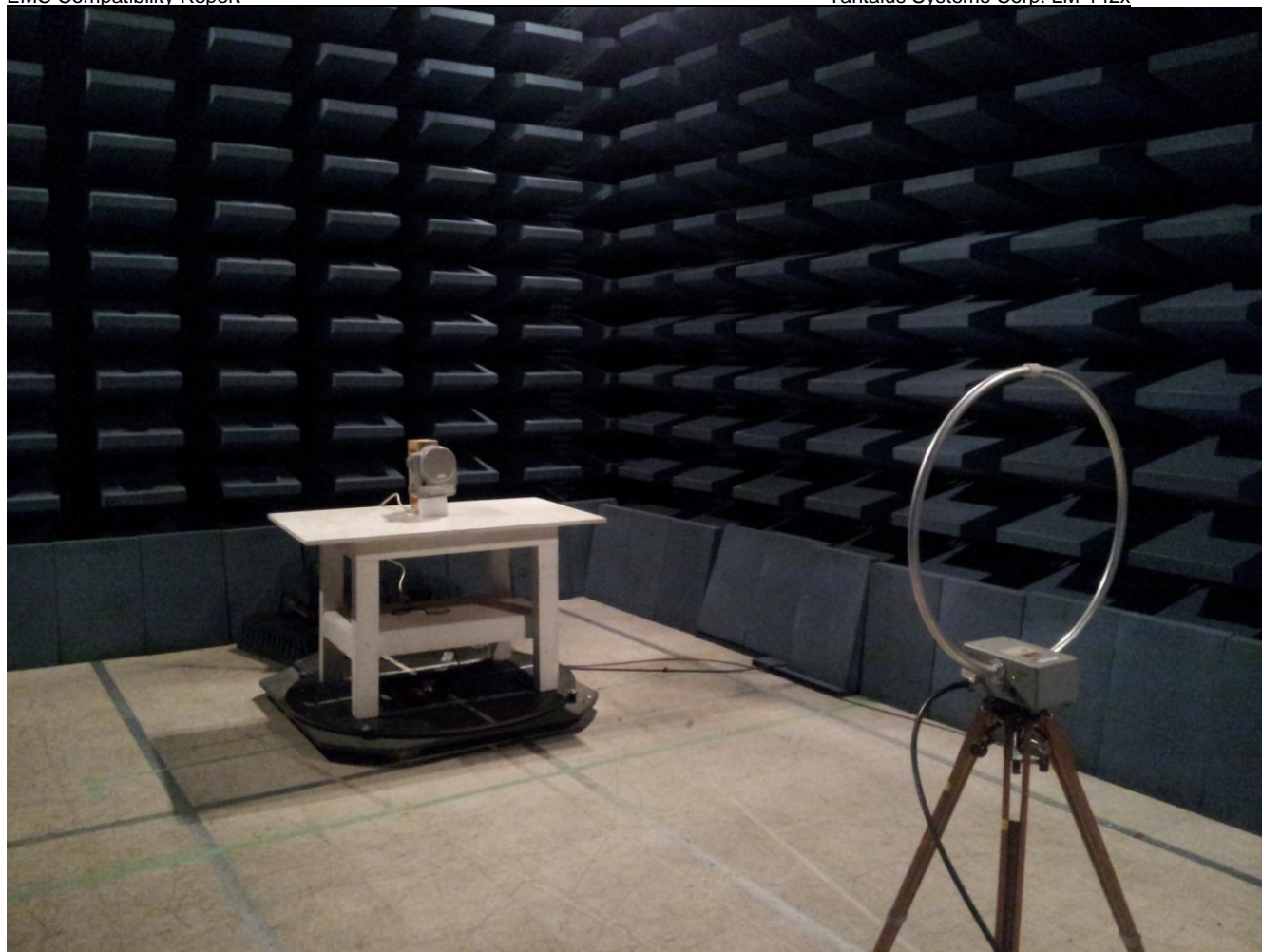
Figure 20: Emissions Test Setup – Intentional / Unintentional Radiated Emissions
