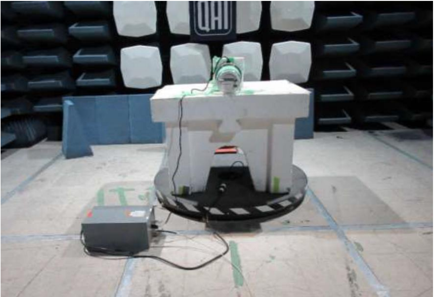
AC conducted Emissions Test Setup
