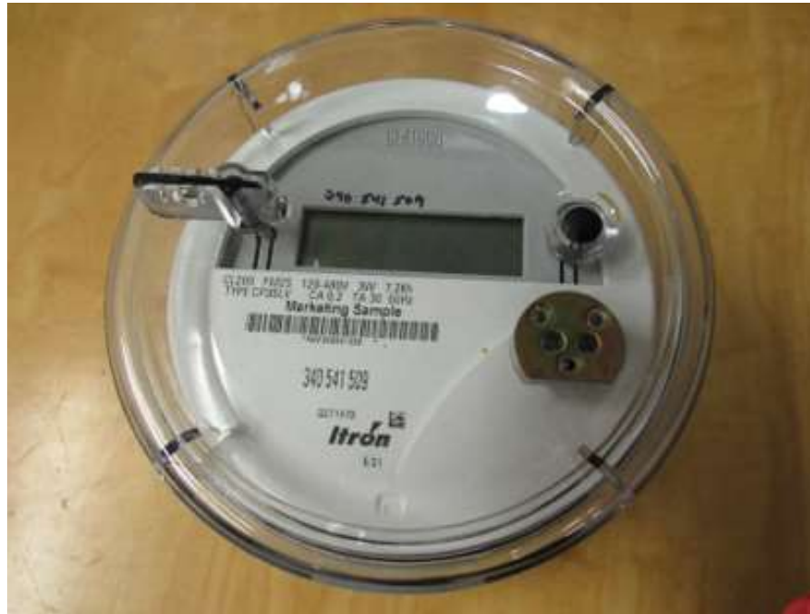
EUT: Itron Electrical Polyphase Meter
