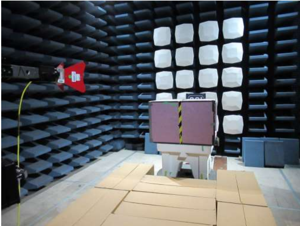
Figure 3: Radiated Emissions performed at the SAC Test Setup, above 1 GHz
