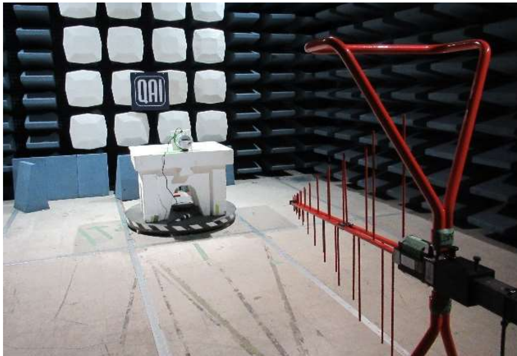
Figure 2: Radiated Emissions performed at the SAC Test Setup, 30MHz to 1GHz
