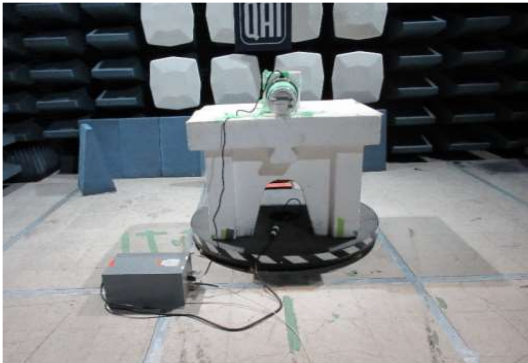
Figure 4: Conducted Emissions performed at the SAC Test Setup
