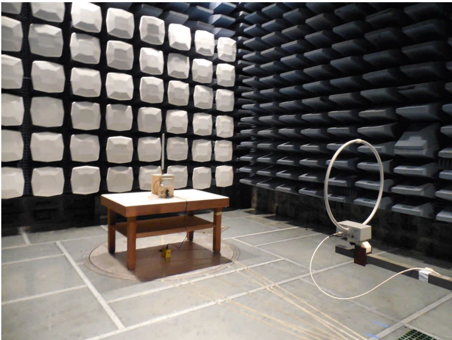
Emissions Test Setup – Intentional/Unintentional Radiated Emissions 0.009 – 30 MHz
