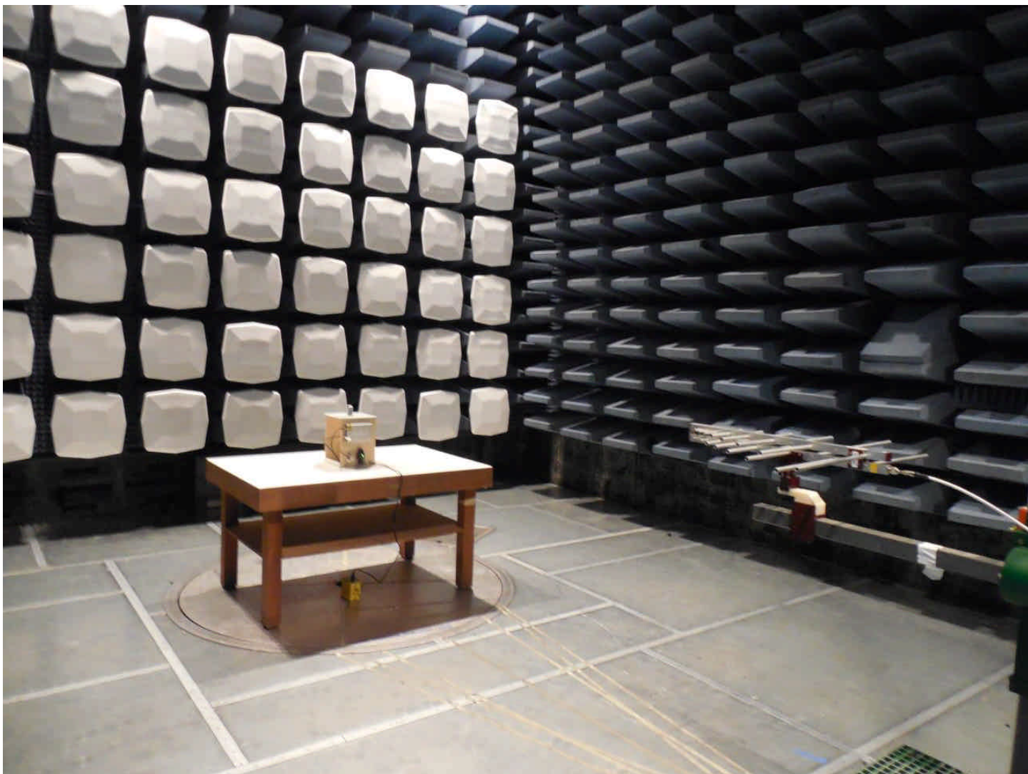
Emissions Test Setup – Intentional/Unintentional Radiated Emissions 30 – 1000 MHz
