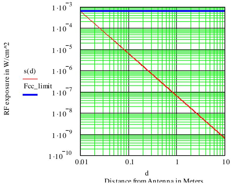
From the graph, it can be observed that the distance at which the RF exposure would exceed the limit would be approx. 10.9cm. The far field distance for a large antenna is given by any distance greater than  $2 D^2 / \lambda$  (where  $D$  is the largest dimension of the antenna); this equates to a minimum distance of 36cm, therefore this calculation is not valid.
