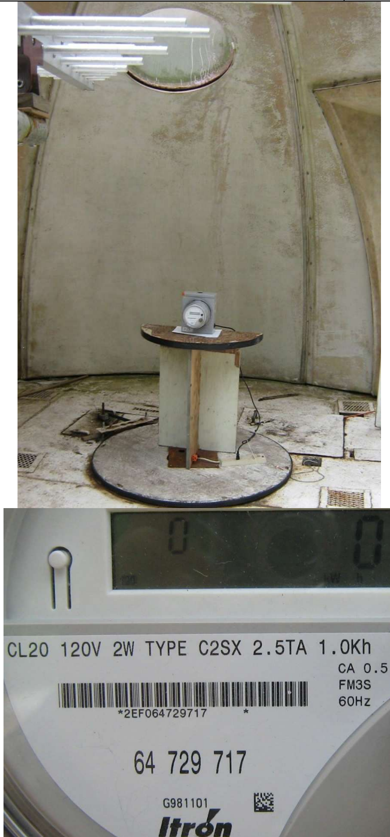
Figure 19: Emissions Test Setup – Unintentional Radiated Emissions, 120V
