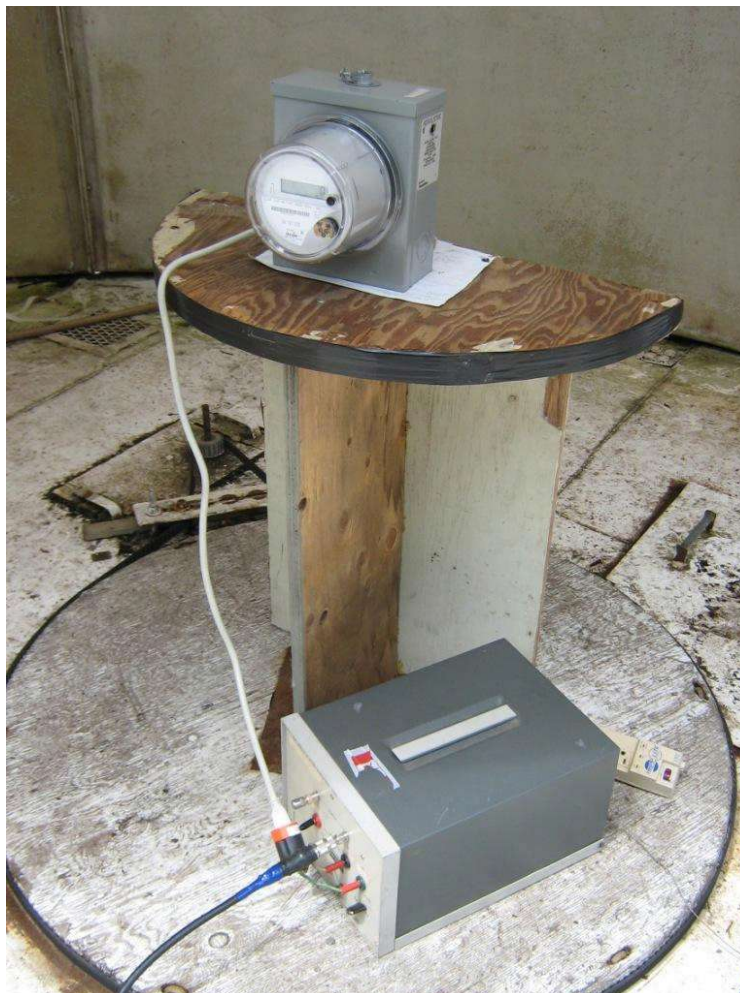
Figure 17: OATS AC Conducted Test Setup
