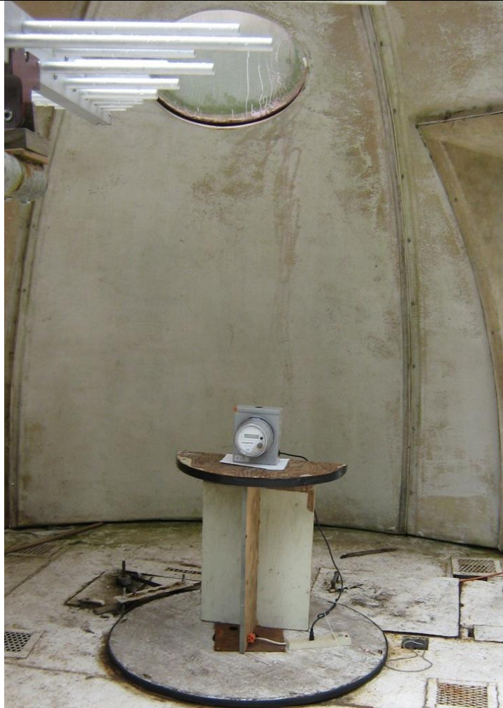
OATS Radiated 200 – 1000 MHz setup.
