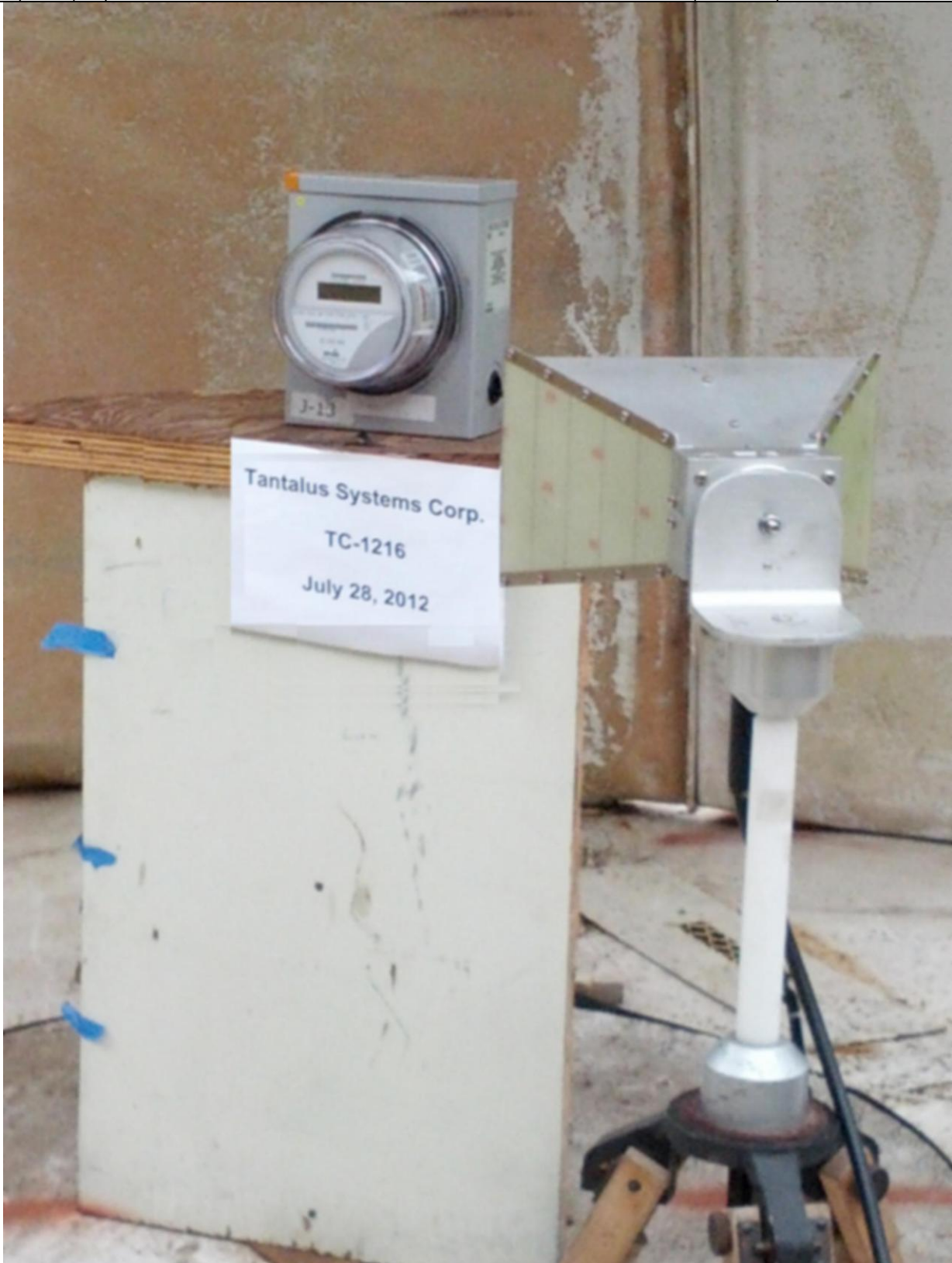
OATS Radiated Intentional 902 – 9280 MHz setup.
