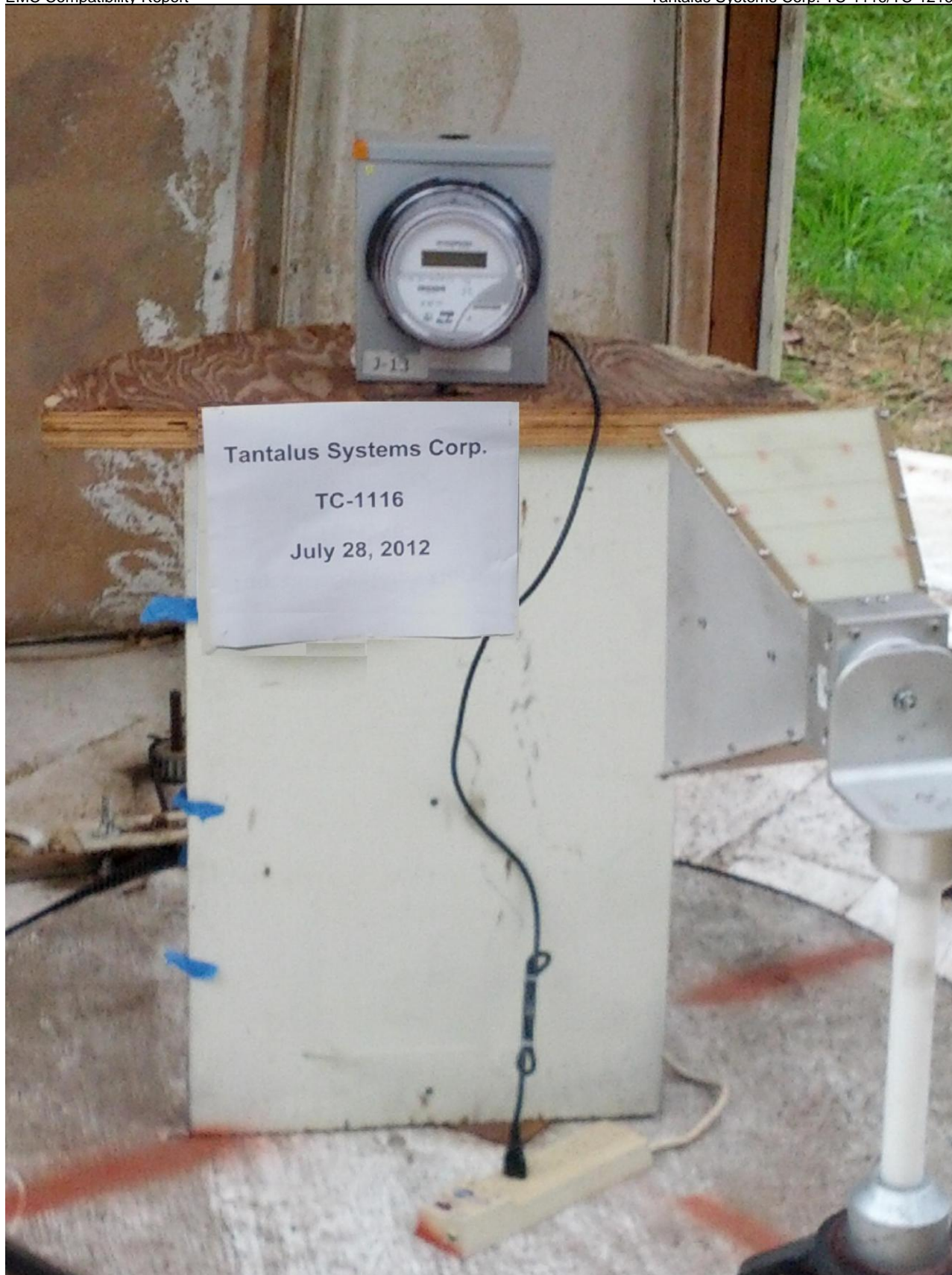
OATS Radiated Intentional 902 – 9280 MHz setup.
