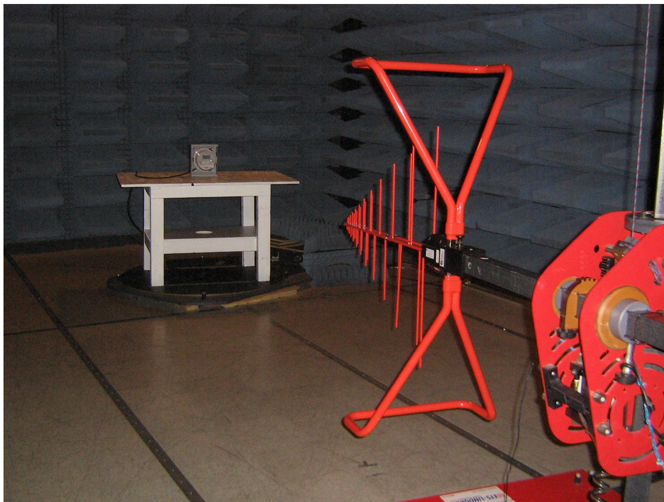
Figure 17: Emissions Test Setup –Radiated Emissions – I-210+ 120V and 240V
