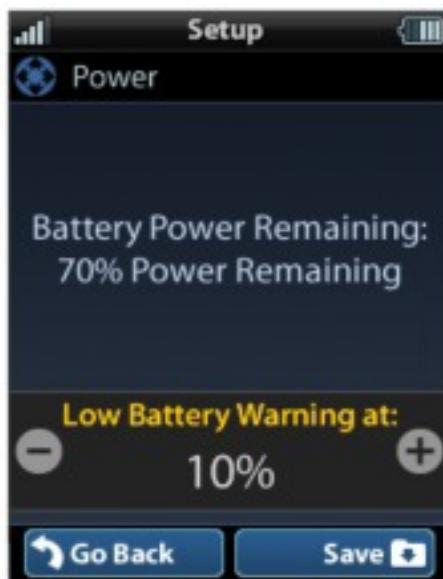
The low battery warning message can be adjusted from this section. Adjust the battery percentage using the “-” and “+” buttons to do so.
