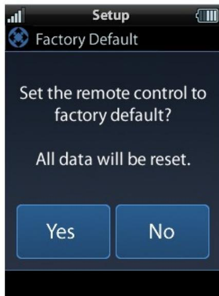
Selecting **Yes** started the factory reset process. This should only be done when instructed by URC Technical Support or by the smart home professional installer.
