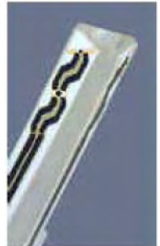
Fig 5. Probe Thick-Film Technique
