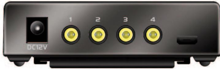
**DC 12V Power:** Plug in the included 12V DC 1A power supply.
