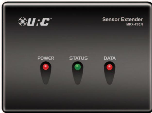
**Power LED:** The Power LED illuminates when the unit is powered.
