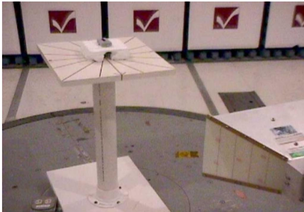
View of the Spray Commander transmitter during the Radiated Emissions tests. This view shows the orientation of the product corresponding to zero degrees azimuth in position. (horizontal polarity).
