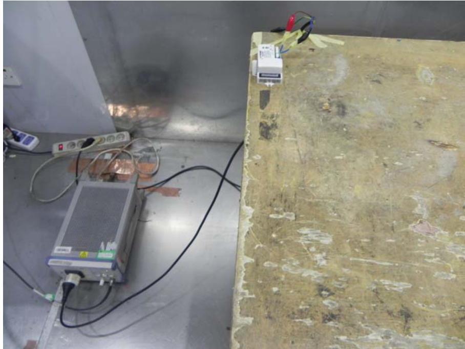
Photograph – Conducted Emission Test Setup
