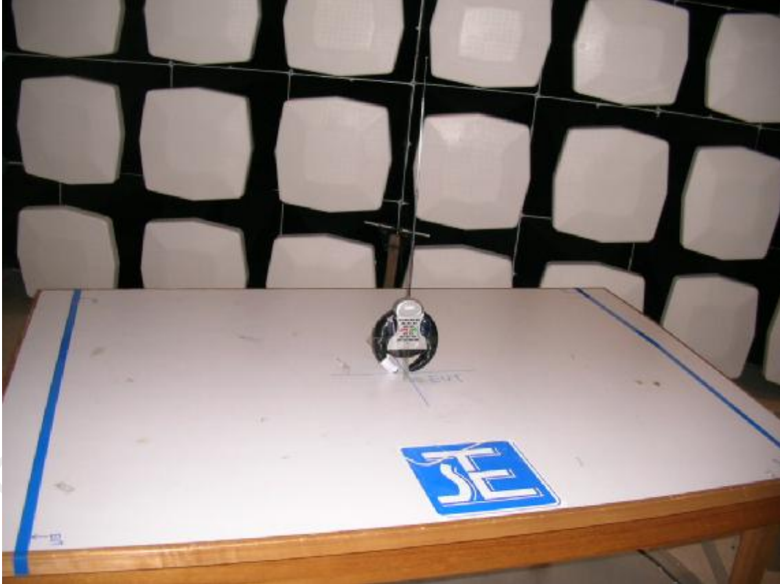
Measurement of Radiated Emission Test Set Up
