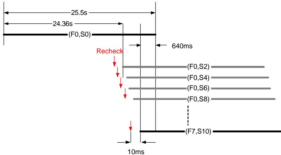
When operating in a quiet radio environment in which  $(F0, S0)$  is always available, the control channel will alternate between  $(F0, S0)$  and  $(F0, S2)$  every  $25s$  and hence the requirements of FCC 15.323 (c) (4) are met. This scenario is shown in the following diagram.
