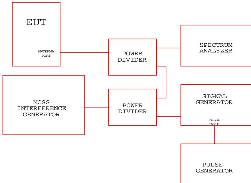
**Test Configuration Block Diagram
