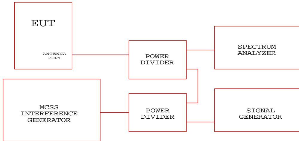
**Test Configuration Block Diagram
