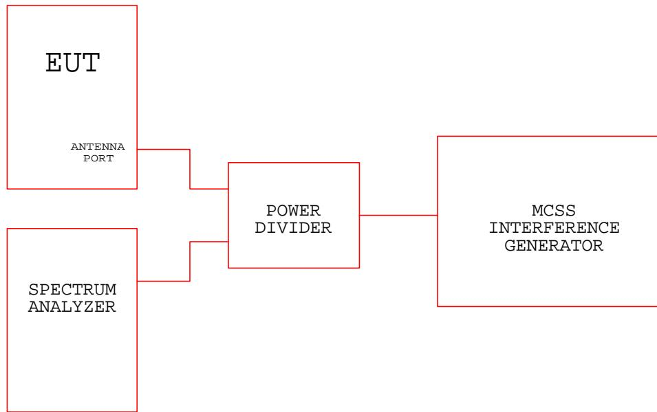
**Test Configuration Block Diagram
