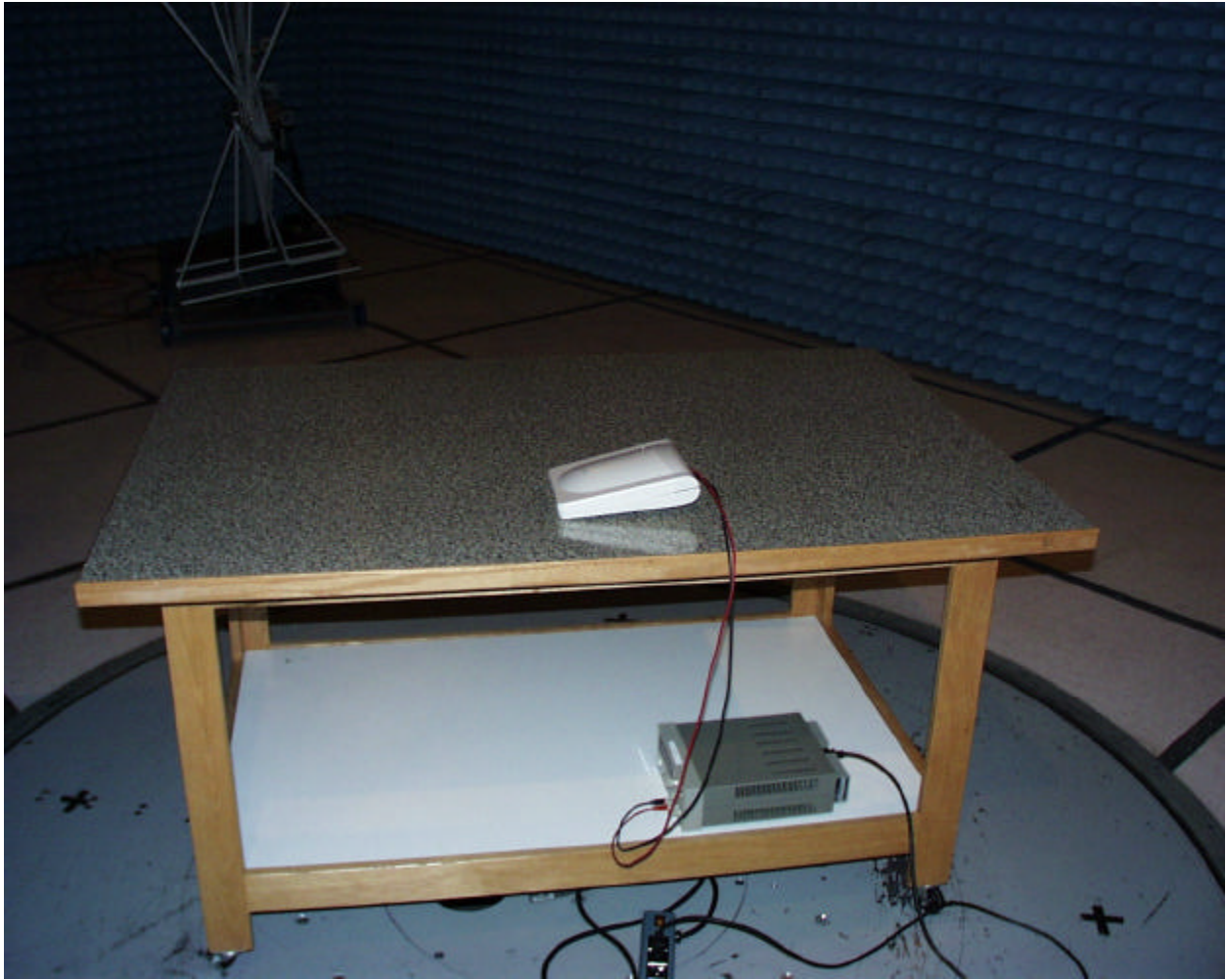
Back View of Worst Case Radiated and Line Conducted Emissions Test Set-up
