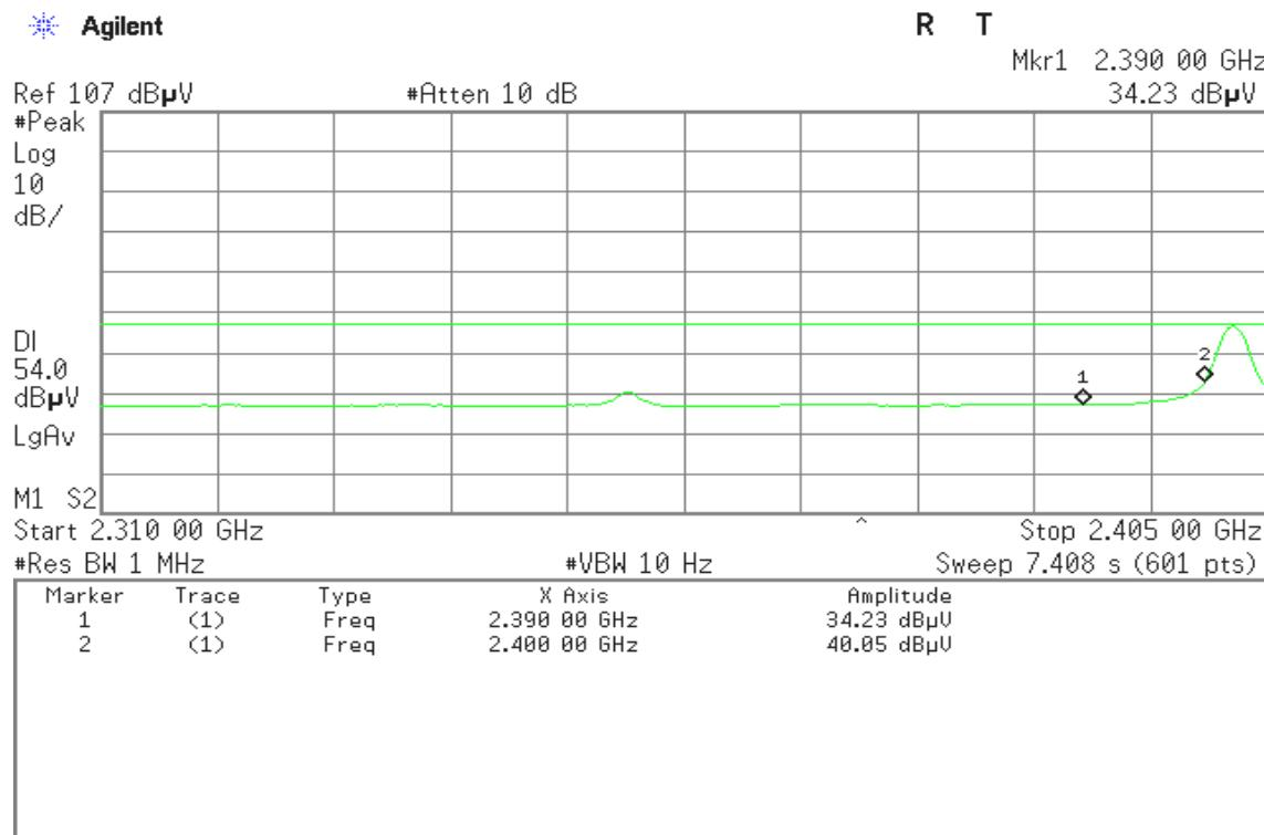
**Band Edges (CH High)****Detector mode: Peak****Polarity: Vertical**
