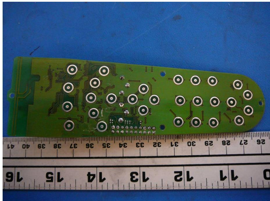
**9.20 LR102 EUT Display Board Component View**
