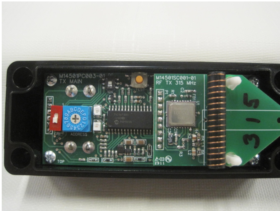
Main and RF in Enclosure
