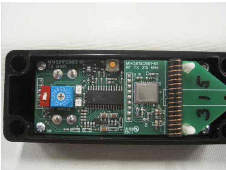
Main and RF in Enclosure
