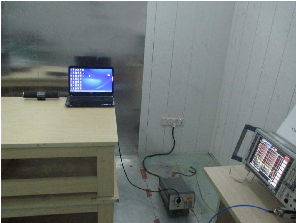
FCC RADIATED EMISSION TEST SETUP
