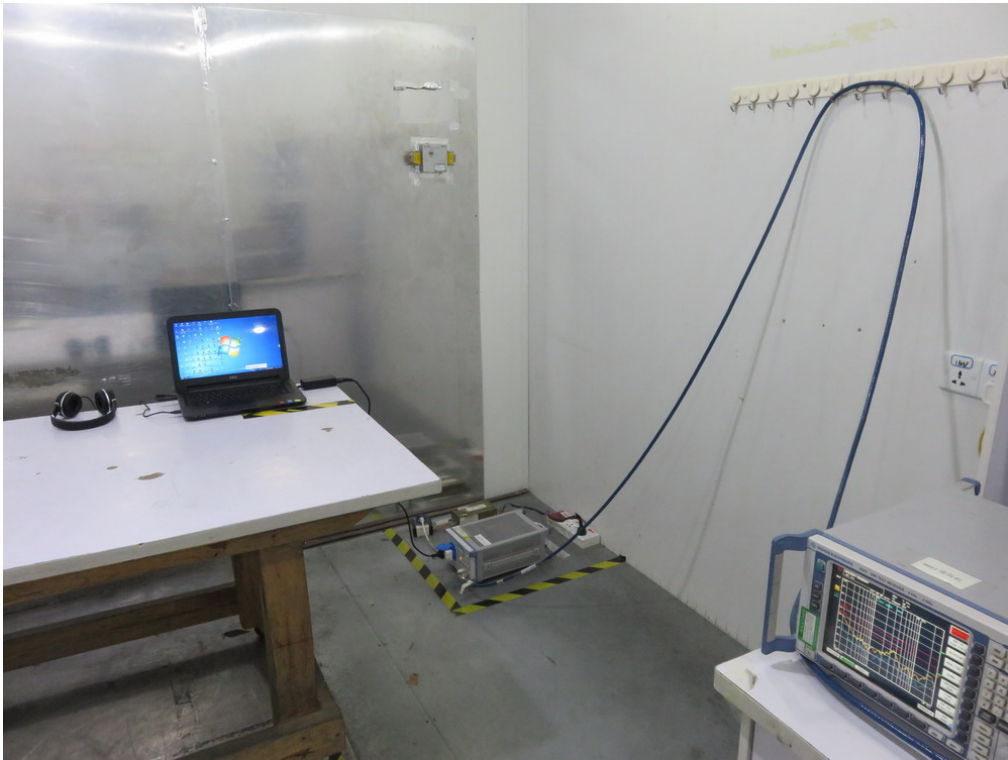
FCC RADIATED EMISSION TEST SETUP
