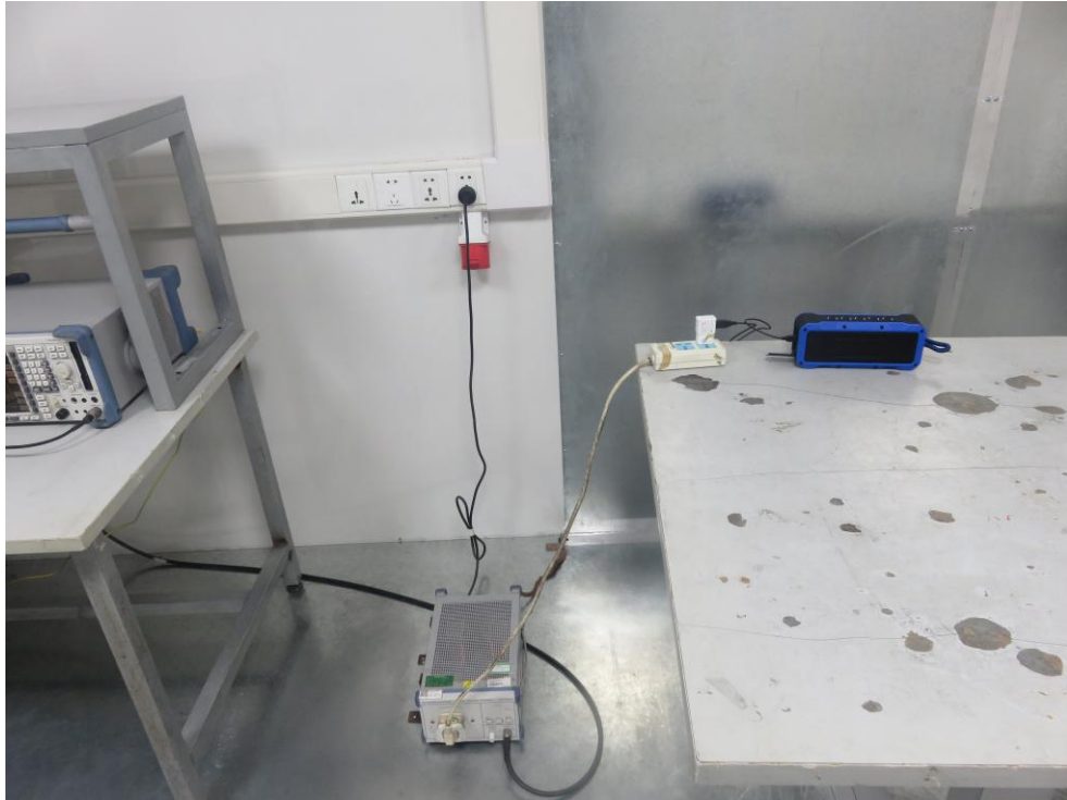
Photo of Conducted Emission Measurement
