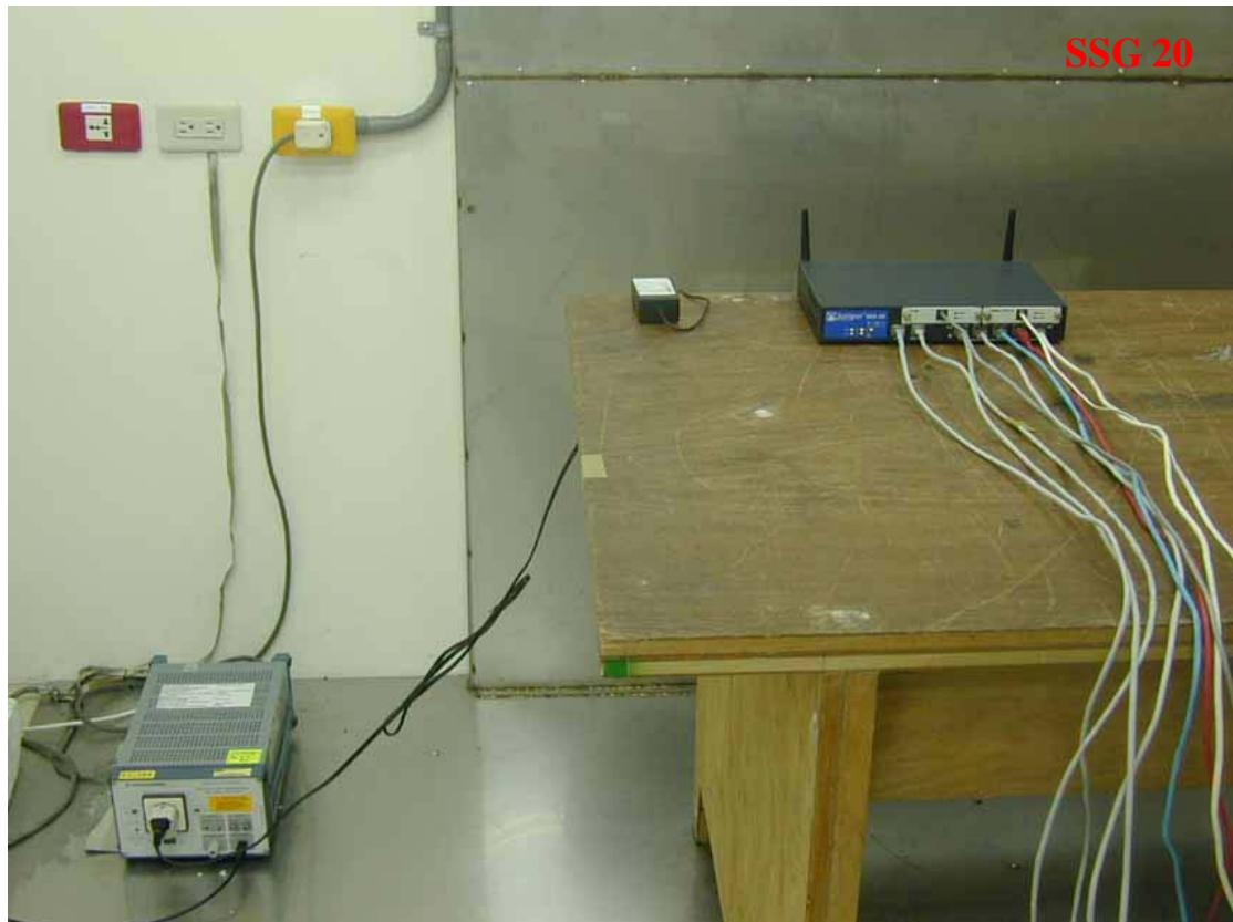
**Photo 4: Conducted Emission Test Set-up photo**
