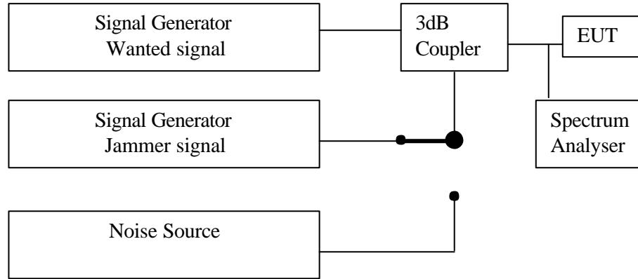
For the test, 50 000 bursts were sent and the level of the Jammer Signal Generator was changed until an ACER level of 0.1% was reached. This was recorded as the J/S ratio.
