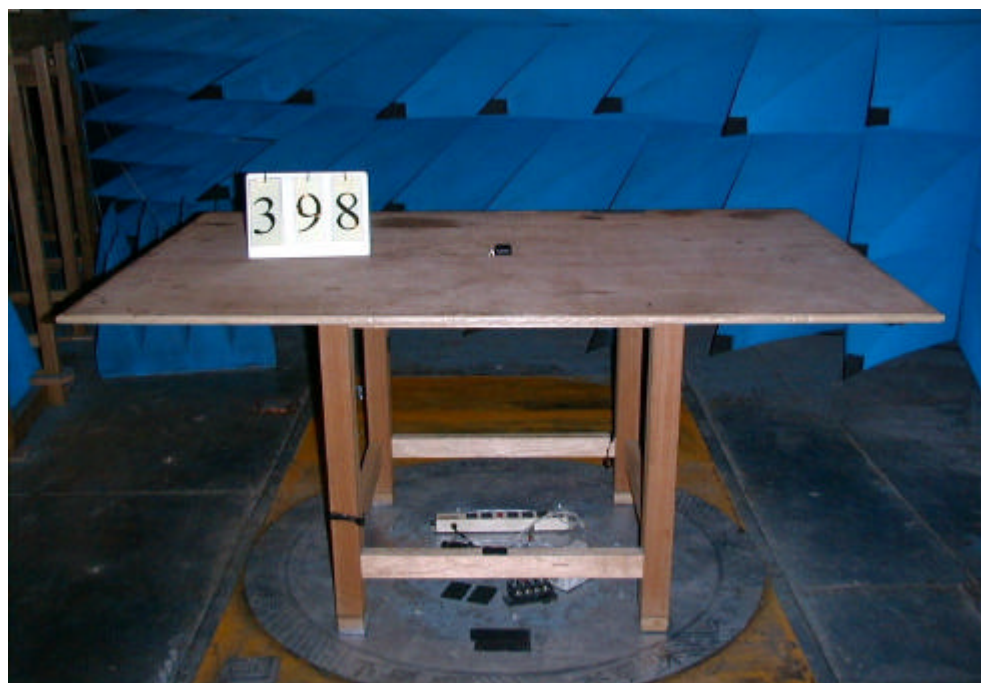
fig 2. Test Configuration of the Radiated Emissions (Back View)
