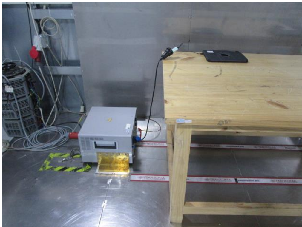
Photograph 2: Set-up for measurement of Conducted Emission, THZ988
