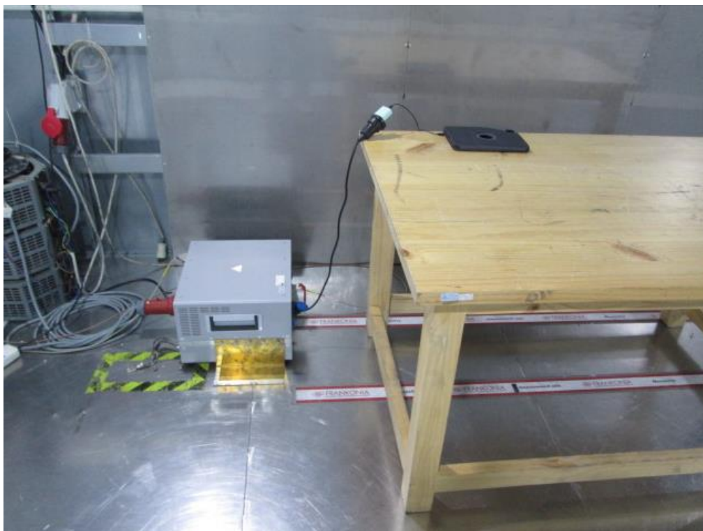
Photograph 4: Set-up photo for Radiated Emission, 30MHz - 1GHz, THZ988
