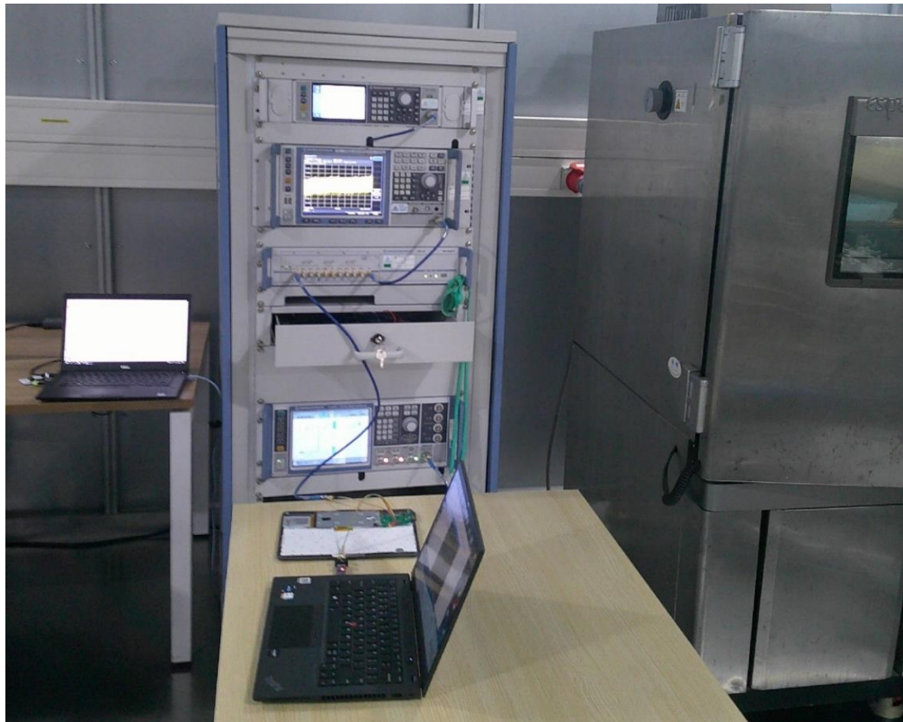
Photograph 2: Set-up for measurement of Conducted Emission, THZ988
