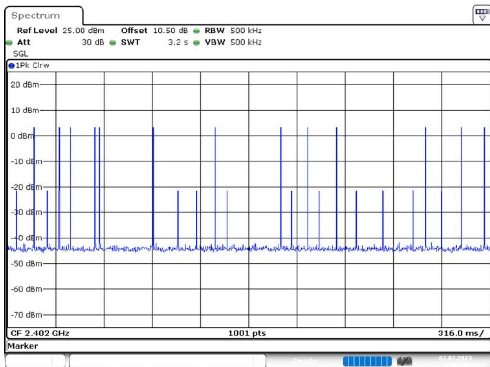
**EDR Mode ( $\pi/4$ -DQPSK)****2DH1: Pulse Width**
