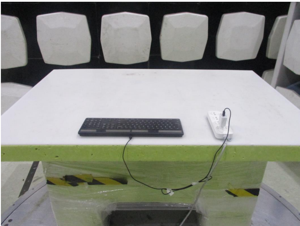
Below 1GHz The EUT is placed at the center of turntable
