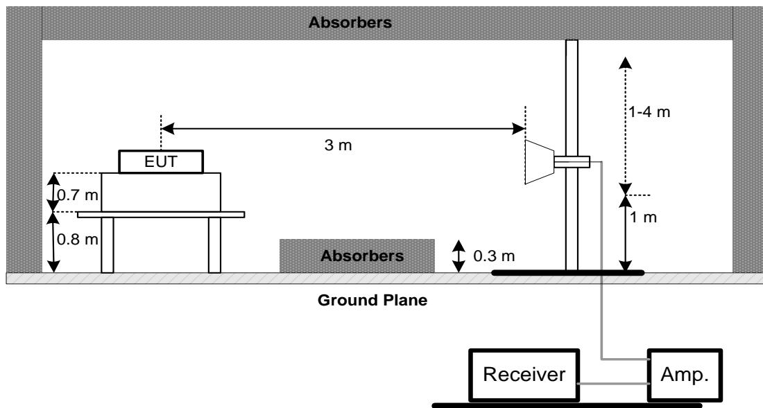
(C) For Radiated Emissions Below 30MHz
