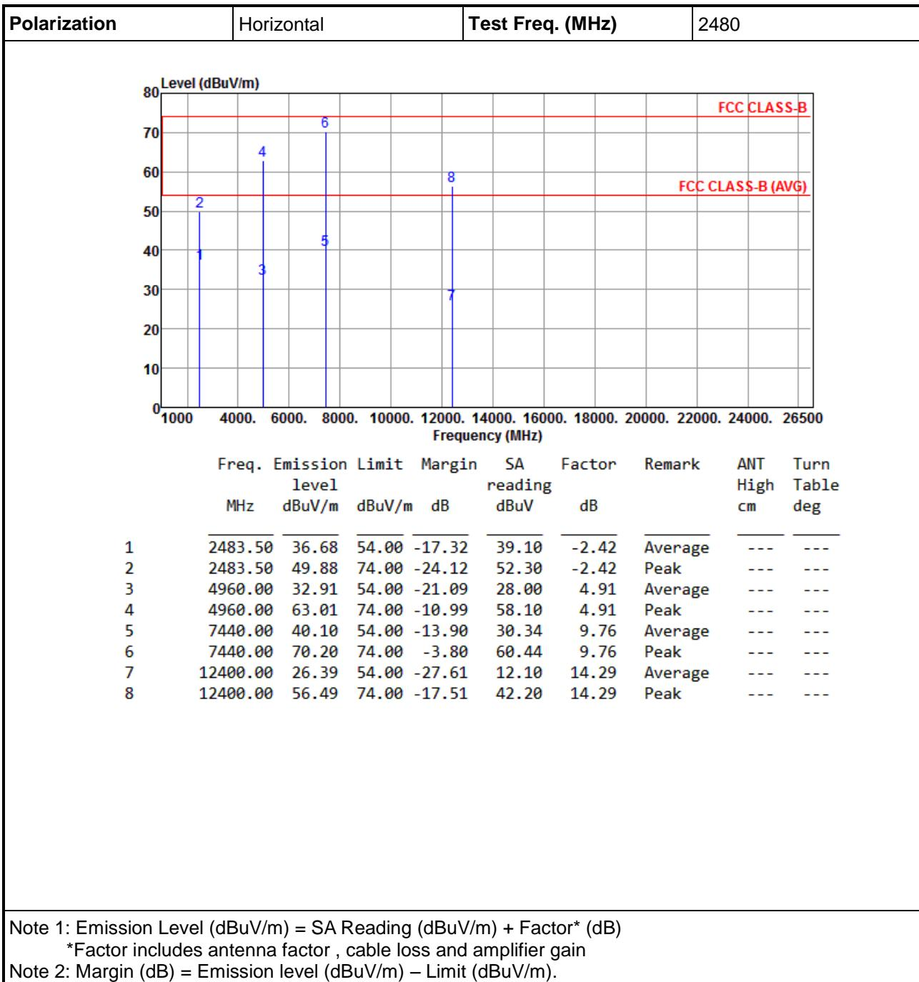
Note 1: Emission Level (dBuV/m) = SA Reading (dBuV/m) + Factor\* (dB)
