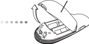
Insert the supplied batteries, making sure the positive (+) and negative (-) ends of the batteries match the polarity indicators inside the battery compartment.
