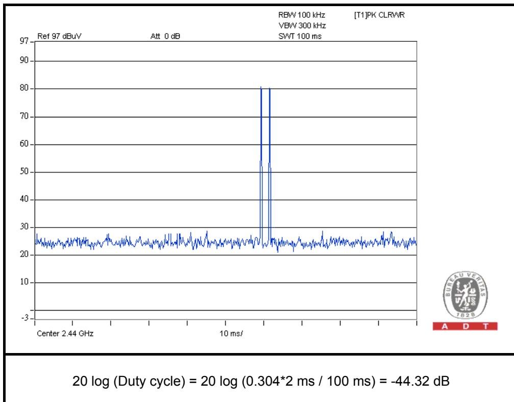
$$20 \log (\text{Duty cycle}) = 20 \log (0.304 * 2 \text{ ms} / 100 \text{ ms}) = -44.32 \text{ dB}$$
