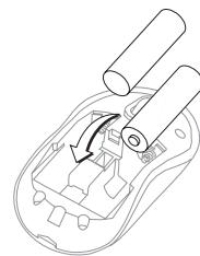
5. Replace the battery safety clip by sliding it forward until it clicks into place and then replace the battery cover.
