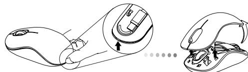
2. Remove the battery safety clip by squeezing the center of the clip and sliding it back, towards the rear of the mouse. Lift up and rotate the clip out of the way.
