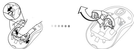
3. Remove the micro USB receiver stored inside the center compartment .
