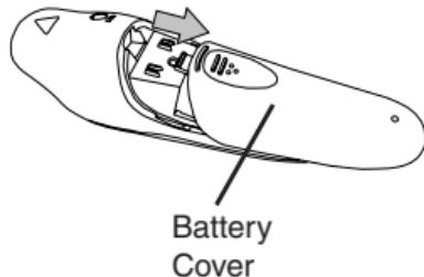
Insert the supplied battery, making sure the positive (+) and negative (-) ends of the battery match the polarity indicators inside the battery compartment.
