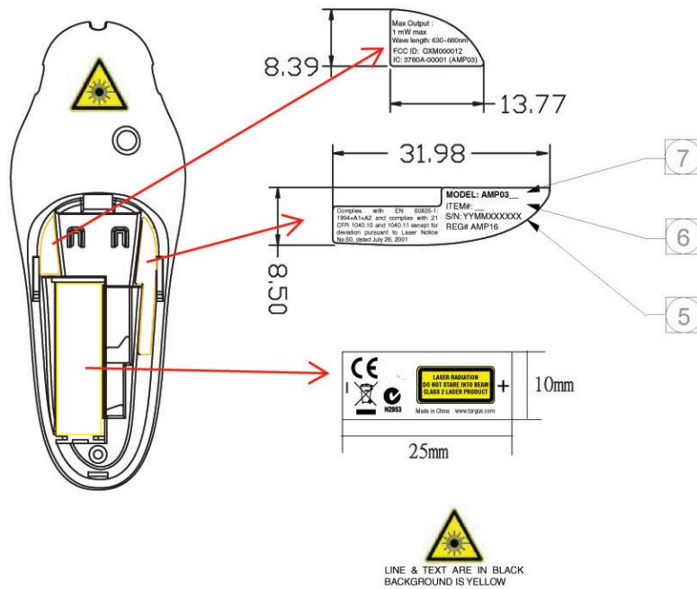
8. The FCC identifier is located inside the battery compartment and will also appear on the box.
