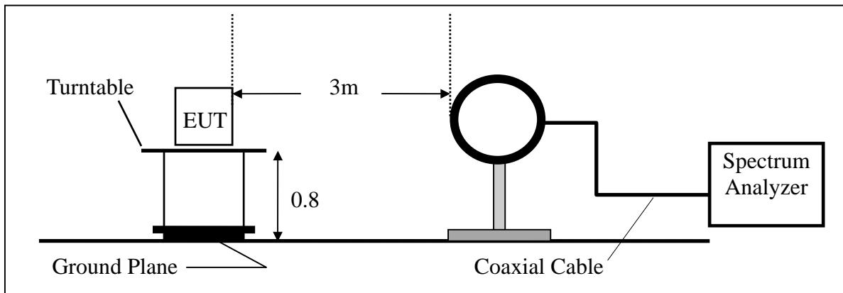
**For Frequencies below 1 GHz**
