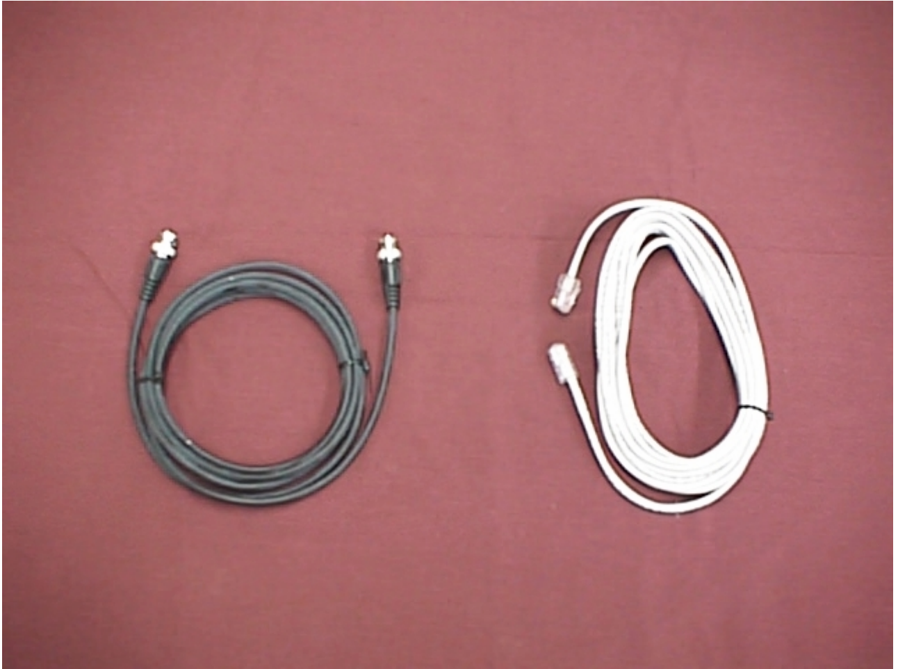
Figure 3-4 10Base2 (left) and 10BaseT (right) Ethernet Cables
