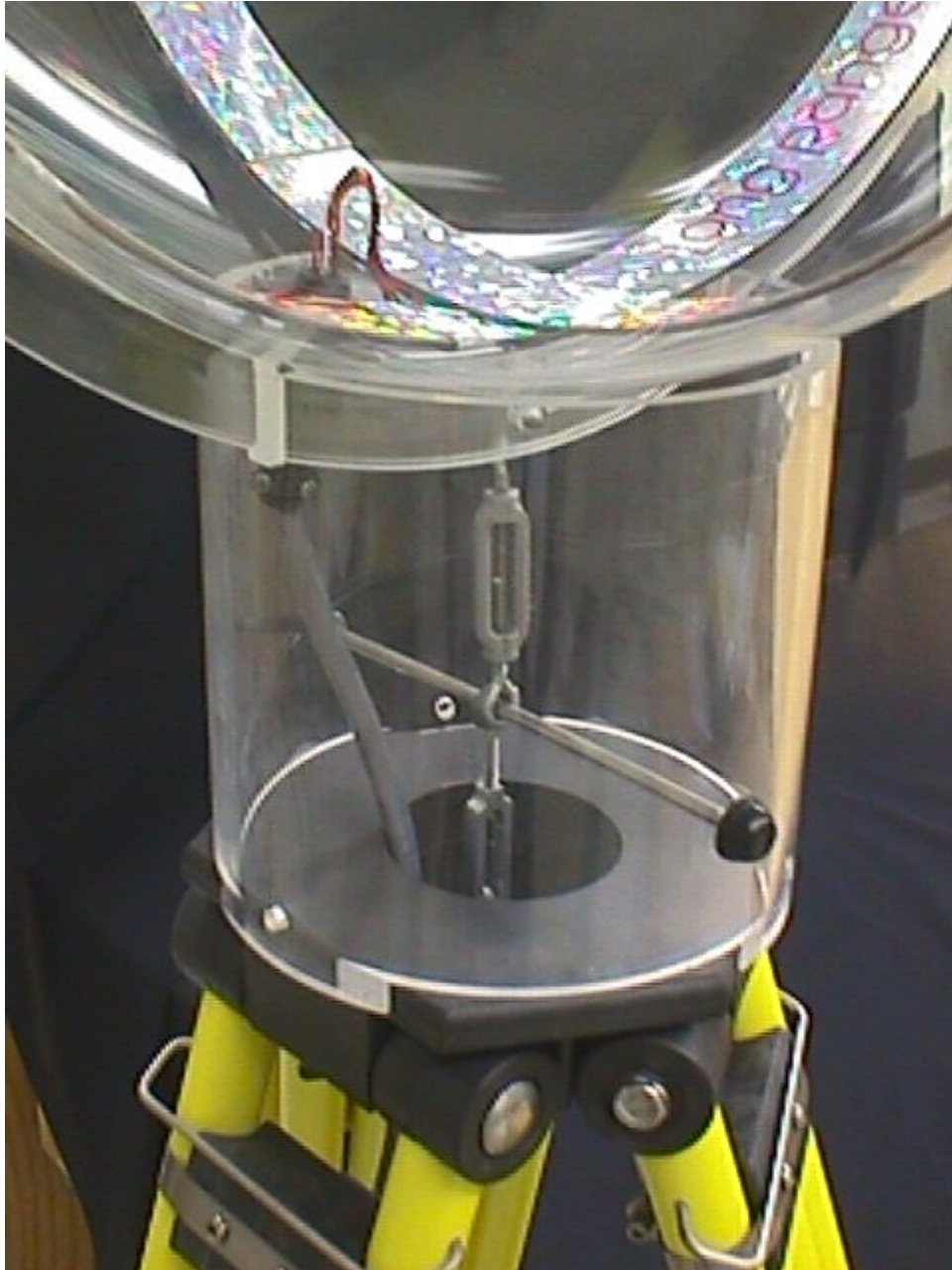
Figure 4-5 Long Ranger Transmitter Mounting Structure
