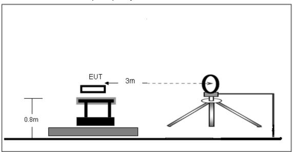
(B) Radiated Emission Test-Up Frequency 30MHz~1GHz
