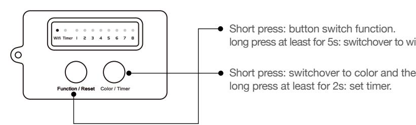
(2-1) Press the Color/Timer button and hold for more than 2 seconds, you can set the timer. When timer is working, the green timer indicator will light up.
